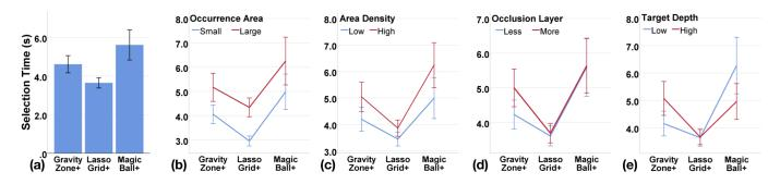
Fig. 8. Plots of selection time for the three improved techniques. These plots include techniques' overall selection time (a) and their selection time in different levels of Occurrence Area (b), Area Density (c), Occlusion Layer (d), and Target Depth (e). Error bars indicate the 95% confidence interval.
