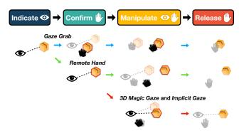
Figure 1: An illustration of the target manipulation process, where gaze is used for indicate, hands are used for trigger confirm and release, and both inputs are applied (as hand only, or gaze and hand collaboratively) for object manipulation.
