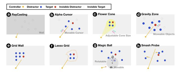
Fig. 3. The RayCasting technique (a) and techniques devised for fully-occluded target selection, including Alpha Cursor (b), Flower Cone (c), Gravity Zone (d), Grid Wall (e), Lasso Grid (f), Magic Ball (g), and Smash Probe (h).
