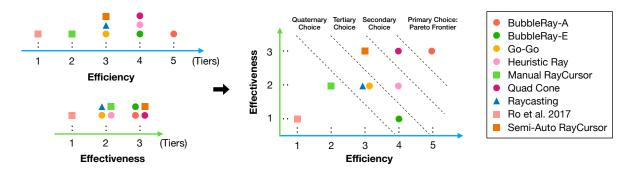
Fig. 9. To maximize performance measures (i.e., efficiency and effectiveness), we placed all the candidate techniques onto a 2D plot with efficiency as the x-axis and effectiveness as the y-axis. We can compute Pareto Frontier to determine the most optimal solution (i.e., *BubbleRay-A* in this case). The secondary, tertiary, and quaternary choices can also be concluded.
